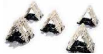
Lux membranes folded into triangular prisms are remarkably strong structures which hold their shape.
