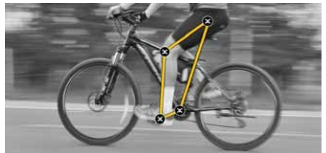
When we ride a bike, we are participating in being a part of a four-bar linkage. The bars are the shaft from the pedal sprocket to the seat, the upper leg, and the pedal shaft. The linkages are the joints in our legs and the bike.
